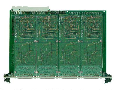
The VME393 32-Channel Differential Input ADC VMEbus Board is very well suited to be used in applications in which autonomous signal conversion is an issue, as well as in standard mid-range applications. Enabled channels are scanned at maximum rate and conversion results are stored in shared memory. Input channels are grouped into 4 sections of 8 inputs each. Each section features a local DSP which performs all functionality and user specific functions can be added for customized operation.
