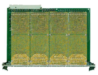
The VME390 features 24 two, three or four wire high-accuracy PT100 measurement channels. Each channel has programmable alarm limits on which an interrupt can be issued. Quad. local DSPs (TMS320C203) perform linearization, auto-calibration and alarm-limit checking. Sensor-data is available in  $\ddot{\imath}$   $\dot{\imath}$   $\dot{\imath}$   $\dot{\imath}$  F, K and Ohms. All inputs are optically isolated from the system.
