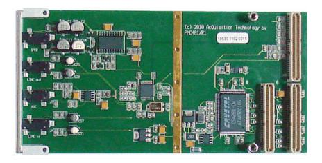
A PMC audio card with front and rear I/O based on the Crystal CS4281 CrystalClearTM PCI Audio Interface controller and the Crystal CS4299 CrystalClearTM SoundFusionTM Audio Codec '97. The PMC481 features four audio connections via the front panel using 3.5mm stereo connectors.
