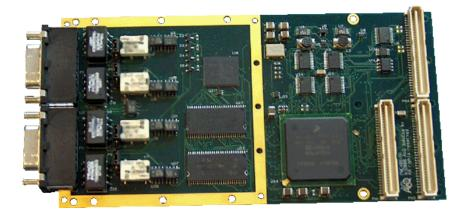
An intelligent quad channel CAN controller PMC, suitable for the standard CAN2.0B, but also for the CAN aerospace, ARINC-825 protocol.
