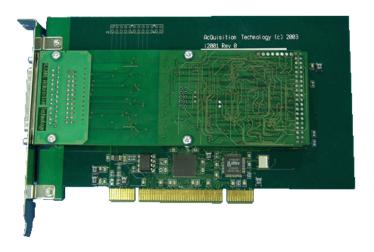
The PCI385 Universal Timer Counter PCI card is an ideal solution for automated test and measurement applications. The PCI385 features two timer/counter inputs. Both inputs have a coaxial connector for the input range of +/- 10 V and high-voltage pins for the input range of +/- 300 V. The coupling of the inputs is either AC or DC. The PCI385 provides 6 measurement functions: frequency, high-time, low-time, period, counter and phase measurements.
