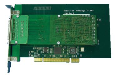
The PCI323 Quadrature Incremental Encoder Interface is designed to interface with up to six quadrature incremental encoders. This is an ideal solution for all applications where several encoders must be connected with a maximum of flexibility and a minimum of overhead.
