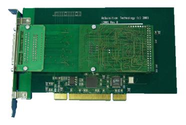
The PCI322 Intelligent Stepper Motor Controller is designed to drive external amplifiers. This is an ideal solution for all applications where stepper motors must be controlled with a maximum of flexibility and a minimum of overhead. The local processor handles all high-level commands to provide maximum control for both straightforward as very complex applications
