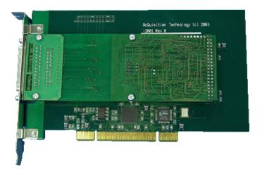
The PCI302 provides four ARINC-429 compatible channels (2x receive and 2x transmit) at any rate between 12.5 and 100kbps.
