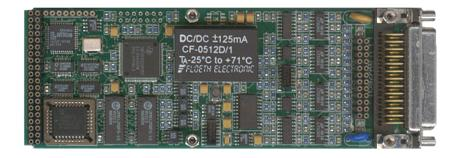
The M392 16-Channel Common-Mode Input ADC m-module is very well suited to be used in applications in which autonomous signal conversion is an issue, as well as in standard mid-range applications. A local TMS320C203 DSP provides processing capabilities to scan all enabled channels at a programmable rate, perform gain/offset compensation and store conversion results in dual ported memory.
