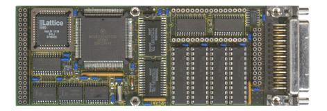
The M312 General Timing Analyser/Synthesizer M-module has an MC68332 CPU. The MC68332 contains intelligent peripheral modules such as the time processor unit (TPU), which provides 16 microcoded channels for performing time-related activities from simple input capture or output compare to complicated motor control or pulse width modulation. All 16 TPU channels and 4 general purpose I/O channels are buffered and available on the connector for use with for instance an external amplifier.
