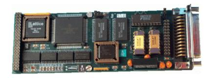
The M302 ARINC-429 Controller M-module is based upon the popular Motorola MC68332 microcontroller. The TPU of this device has been programmed to handle the ARINC-429 transmit and receive algorithms, while the CPU neatly organizes the traffic between the bus and the host CPU. As the user remains in full control, this provides a versatile and user-friendly ARINC-429 interface.
