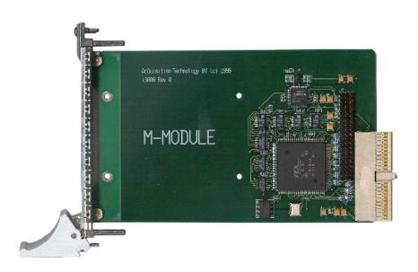
The i3000 M-module Carrier for CompactPCI features a 3U form factor CompactPCI gateway to the M-module interface. One M-module mounting socket is provided by this carrier. This carrier can be used in temperatures from -40°/+85°C. The M-module interface of the i3000 complies to the M-module Specification ANSI/VITA 12-1996. The interface features A8, A24, D16 and D32 access types.
