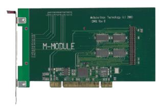
The i2001 M-module Carrier for PCI bus implements a PCI bus gateway to the M-module interface. One M-module mounting socket is provided by this carrier. The M-module I/O connector is accessible through the PCI card bracket.
