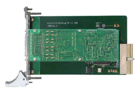
The CPCl392 16-Channel Common-Mode Input ADC card is very well suited to be used in applications in which autonomous signal conversion is an issue, as well as in standard mid-range applications. Enabled channels are scanned at maximum rate and conversion results are stored in shared memory. A local DSP performs the data acquisition and calibration transparent for the host.
