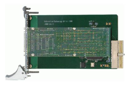
The CPCI302 provides four ARINC-429 compatible channels (2x receive and 2x transmit) at any rate between 12.5 and 100kbps. Because the CPCI302 is built upon a flexible platform, the user functions can be implemented almost without restriction, making this product flexible and user-friendly.
