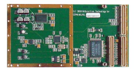
A conduction cooled PMC audio card with rear I/O based on the Crystal CS4281 CrystalClearTM PCI Audio Interface controller and the Crystal CS4299 CrystalClearTM SoundFusionTM Audio Codec '97. The PMC481 features four audio connections via the front panel using 3.5mm stereo connectors.
