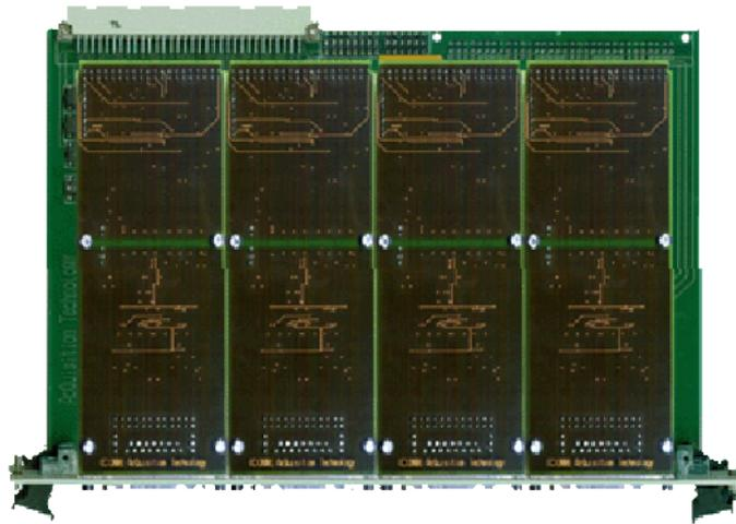
The VME385 Universal/Timer Controller VMEbus board is an ideal solution for automated test and measurement applications. The VME385 features eight timer/counter inputs, all inputs have an coaxial connector for the input range of +/- 10 V and high-voltage pins for the input range of +/- 300 V. The coupling of the inputs is either AC or DC. The VME385 provides 6 measurement functions: frequency, high-time, low-time, period, counter and phase measurements.
