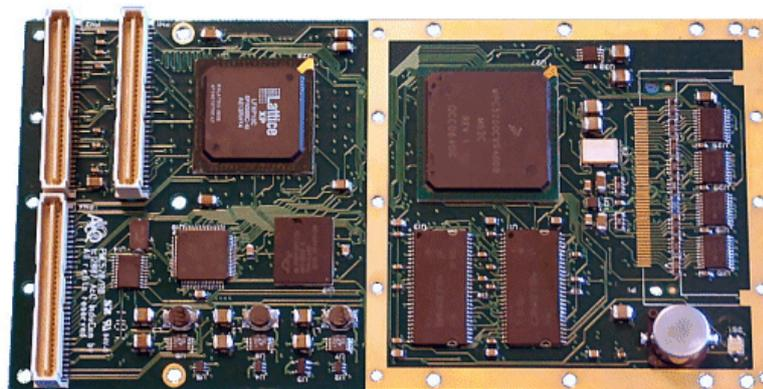
The PrPMC is an MPC5200 based processor PMC. It is the heart of the Low Power Data Acquisition System (LpDAS), but it can also be used as a standard PMC on a PMC carrier card.
