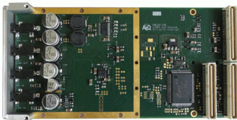
An 8 channel PMC audio card with front and rear I/O for use in embedded computer applications based on the Cmedia CMI8768. This is a single-chip PCI audio controller with integrated codec, full duplex 8 channel DAC and 2 channel ADC, 96k/16bit playback and 48k/16bit recording support.
