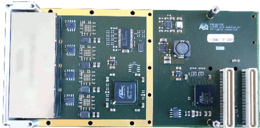
A quad (4-port) 10/100/1000 Mbit Ethernet PMC based controller for use in embedded applications. The PMC401 contains four Intel 82574IT, low power single port Gigabit Ethernet controllers.
