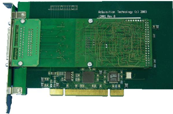
The PCI321 Intelligent Stepper Motor Controller with amplifiers is an ideal solution for all applications where stepper motors must be controlled with a maximum of flexibility and a minimum of overhead. The local processor handles all high-level commands to provide maximum control for both straightforward as very complex applications.
