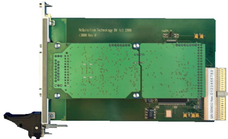
The CPCI385 Universal Timer/Counter CompactPCI card is an ideal solution for automated test and measurement applications. The CPCI385 features two timer/counter inputs. Both inputs have an coaxial connector for the input range of +/- 10 V and high-voltage pins for the input range of +/- 300 V. The coupling of the inputs is either AC or DC. The CPCI385 provides 6 measurement functions: frequency, high-time, low-time, period, counter and phase measurements.
